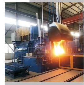
Carbonising and quenching processes ensure to make the mould structure strong and wear resistant.
