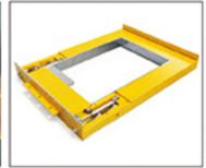
Hydraulic displacement wall The folding wall enables kerbstones with face mix on the surface and side faces.
