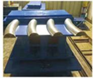
Core puller mould Used for unusual block designs with lateral profiling.
